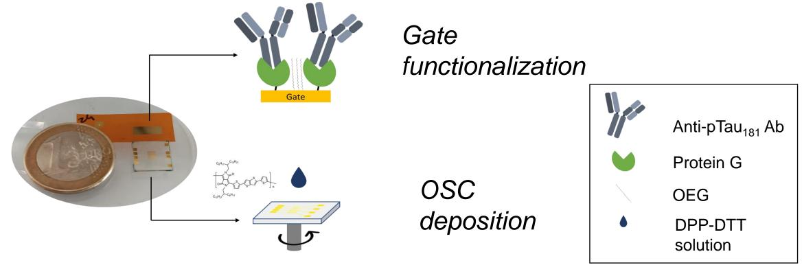
The technology we used as an alternative for the detection of p-Tau is called Electrolyte-Gated Organic Transistors (EGOTs), which have the ability to amplify small biological signals in biological samples, bridging the gap between the biological and technological worlds.<sup>2</sup>
