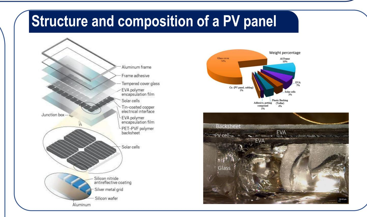
Since October 2022, 9-Tech is performing at pilot scale a thermo-mechanical recycling process to recover from EoL-PVs: glass, aluminium frame, copper ribbons, junction box and PV cells. In the frame of PARSIVAL project, 9-Tech provided to ENEA laboratories small
