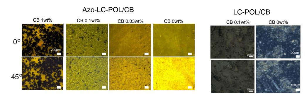
The change of intensity for pristine Azo-LC-POL and its composites with CB wt%<0.1% suggests that in these samples there is the presence of orientational organization.
