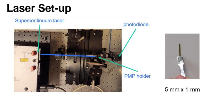
The lasers used are: - 532 nm green DPSS (Diode-Pumped Solid-State) laser - 457nm Solid-State laser - Supercontinuum laser (NKT Extreme)
