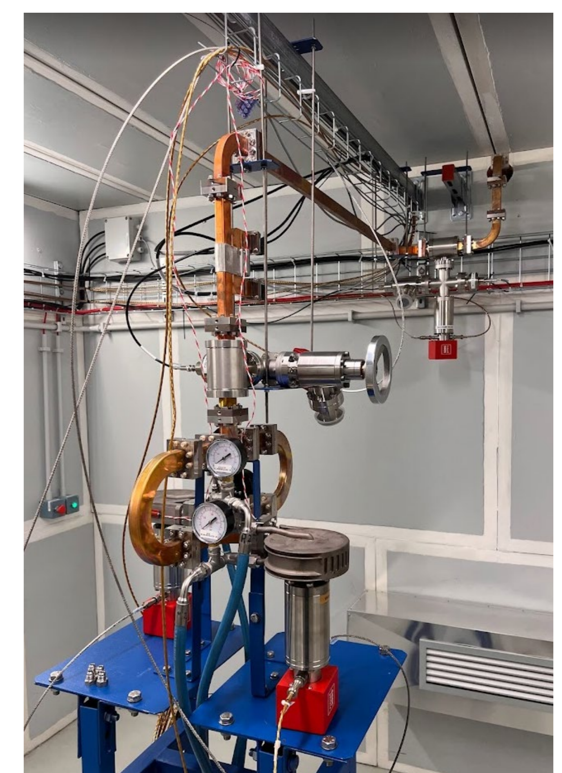
Figure 6: The 3D printed Titanium RF load.
