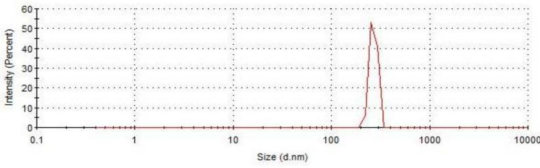
Distribution of droplets function of dimension for the unirradiated emulsion: monomodal distribution at 269.5 nm
