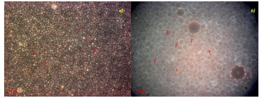
Optical microscopy images of irradiated emulsions: : a) transmission mode, 50X; b) reflexion mode, 100X.
