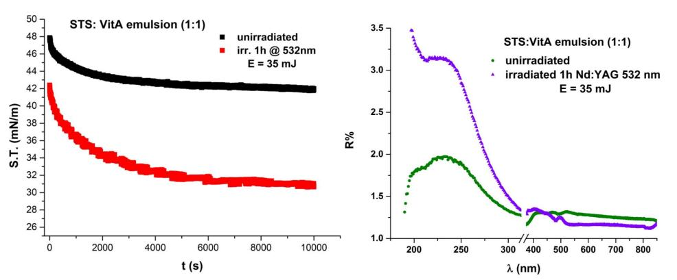
Surface tension comparison of unirradiated and irradiated
