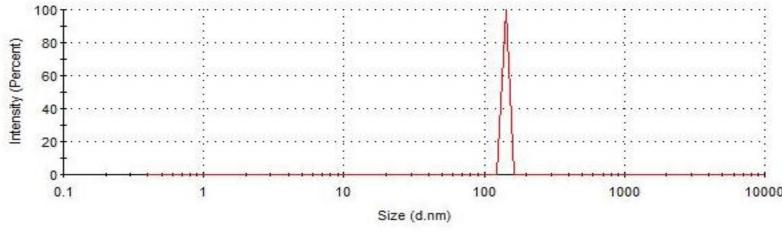
Distribution of droplets function of dimension for the irradiated emulsion: monomodal distribution at 141.8 nm
