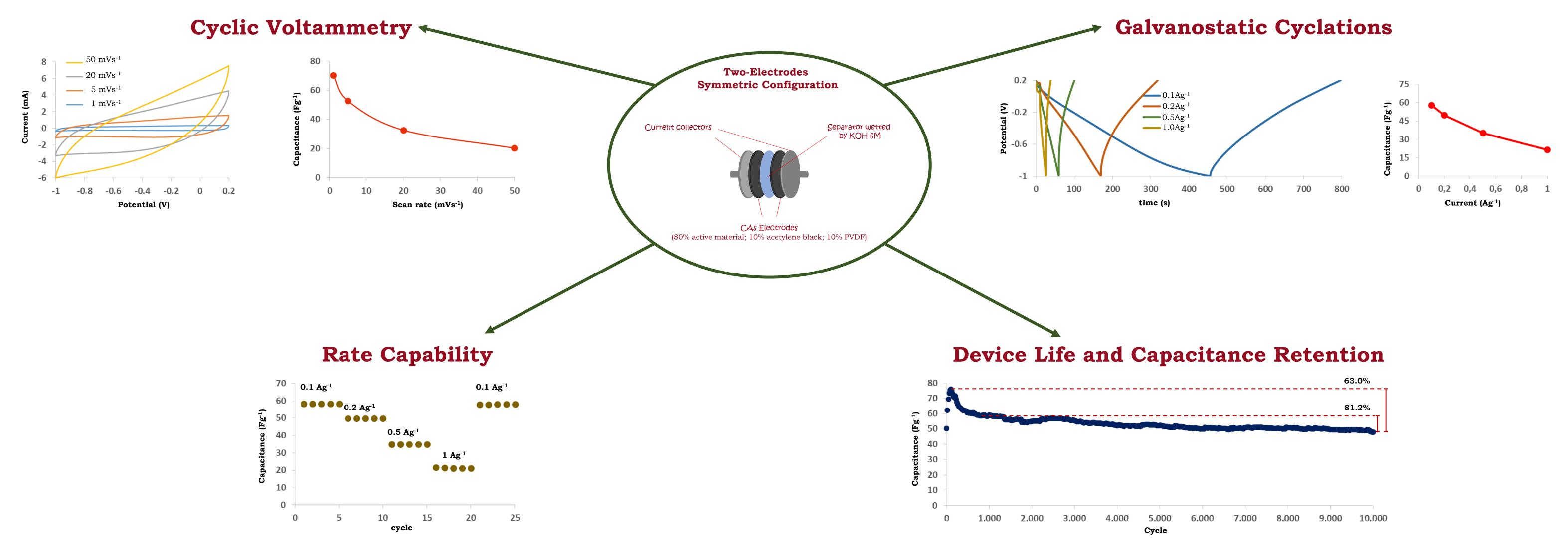
Electrochemical tests on two electrodes symmetrical T-cells show that the CAs have high currents with no peaks during CV and quasi-triangular shape of discharge and charge cycles, which mean CAs have capacitive behaviour. Moreover our material can offer good capacitance with at least 61% of retention after 10'000 cycles, showing long life and resistance over time and under stress condition.
